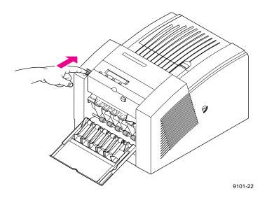
2. Open the exit cover using the blue release button located inside the front cover at the top of the printer.
