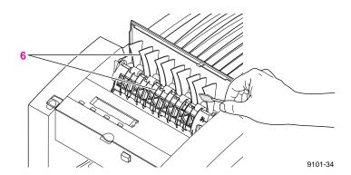
Caution To avoid damaging the print drum and exit guide, never scrape excess ink with a tool or finger nail. Use only the materials provided with the cleaning kit.
