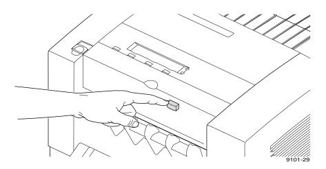
**3.** To clean excess ink particles and drum fluid from the colored exit fingers, gently wipe the top surface of each finger using a *dry* swab.
