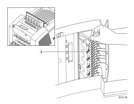
4. To clean the rubber exit rollers, place and hold an alcohol-soaked swab against each roller and turn it several times.
